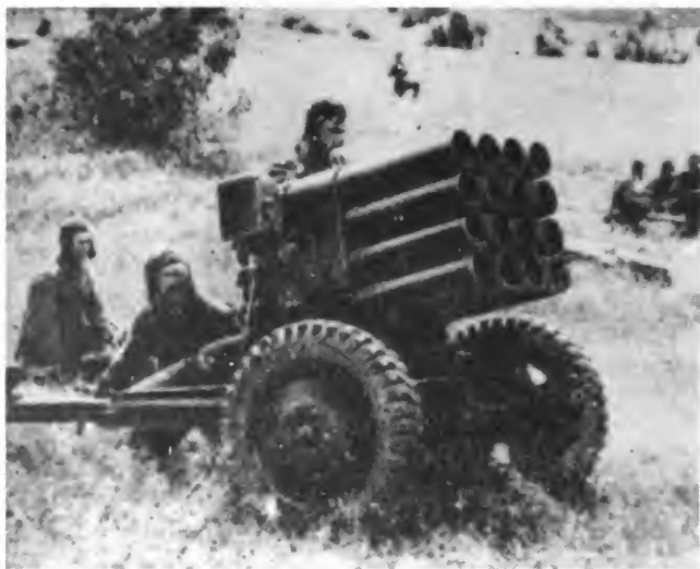
Figure 6-29. Multiple rocket launchers. The 140-mm 16-tube BM-14 (above), towed on a two-wheel carriage, is a standard weapon in airborne divisions. Heavier rockets, such as the 240-mm 12-tube BM-24 (below), are carried on heavy trucks.
